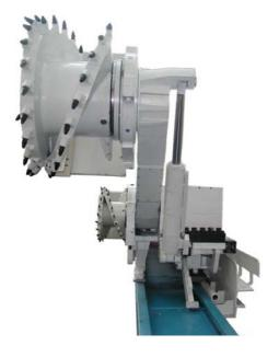
Chassis (1) contains all the elements of the shearer, it is bracket above the panzer conveyor through two skates-guide on the caving side and two skates-support on the face side. The joint of the two skates- guide is through two hydraulic cylinders with double effect in such a way that the machine can tilt towards the face side, in order to be able to follow the coal seam in a line.
