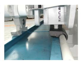
The Hydraulic winch (9) is between both electric motors which is in charge of the movement of the shearer along the mine gallery. This movement is achieved through the traction provided by the motive star of the winch when it engages above a 22 x 66 steel chain placed along the working area and firmly fixed on both sides
