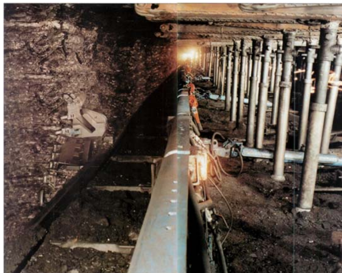
LONGWALL FACE WITH METAL FRAMES
