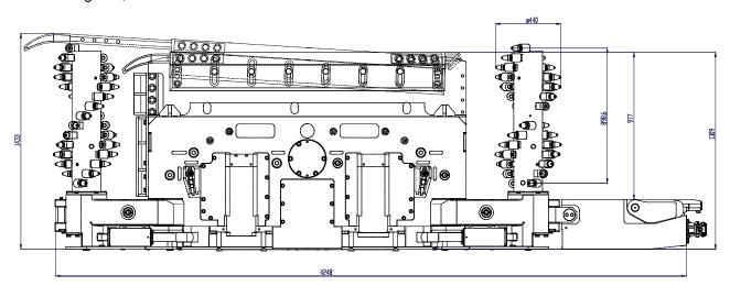
The RPB60 has powered by two electric motors which drive the gear transmission throw the drums located in both sides of the frame
