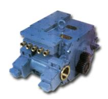
The DC motors (2) type **MU800**, is constructed with steel casing (possibility of anti-flagrant construction in the event of firedamp mines), coupled to the wheel-set by various bronze cushions, thus forming a motor-wheel-set with direct Pinion-Crown transmission to each axle protected with steel casing with a hatch for greasing.
